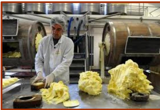
Five vats ferment the cream with a commercial freeze-dried culture at about 22 deg C, slightly higher than Echire for about 48 hours. Beillevaire is not certified to any of the regulatory bodies, so they are not bound by the traditional maturation methods. The cream is then cooled to churn and the process takes about 20 minutes. They wash once to remove buttermilk, which is then sold to a pig farmer for food. They also
