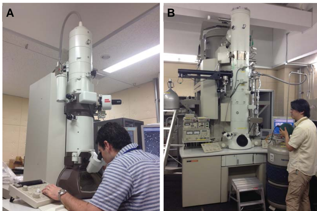
Figure 5: A) Dr Hernan Alonso working with the JEM-1010 and B) Dr Kaoru Mitsuoka filling the JEM-3000SFF with liquid helium.
